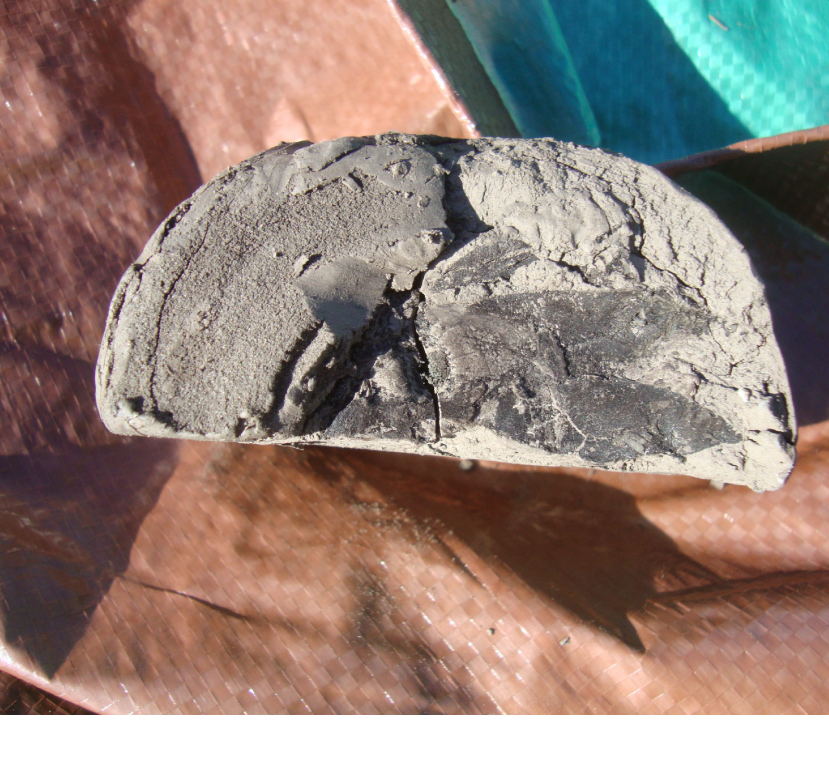
Fossil leaves exposed along a bedding plane from the estuarine to deltaic, palaeobotanical-rich, carbonaceous clays of the Eocene Cockfield Formation from a core of the uppermost beds of the formation. Photographed on November 7, 2012, in Section 19, Township 9 North, Range 3 East.
