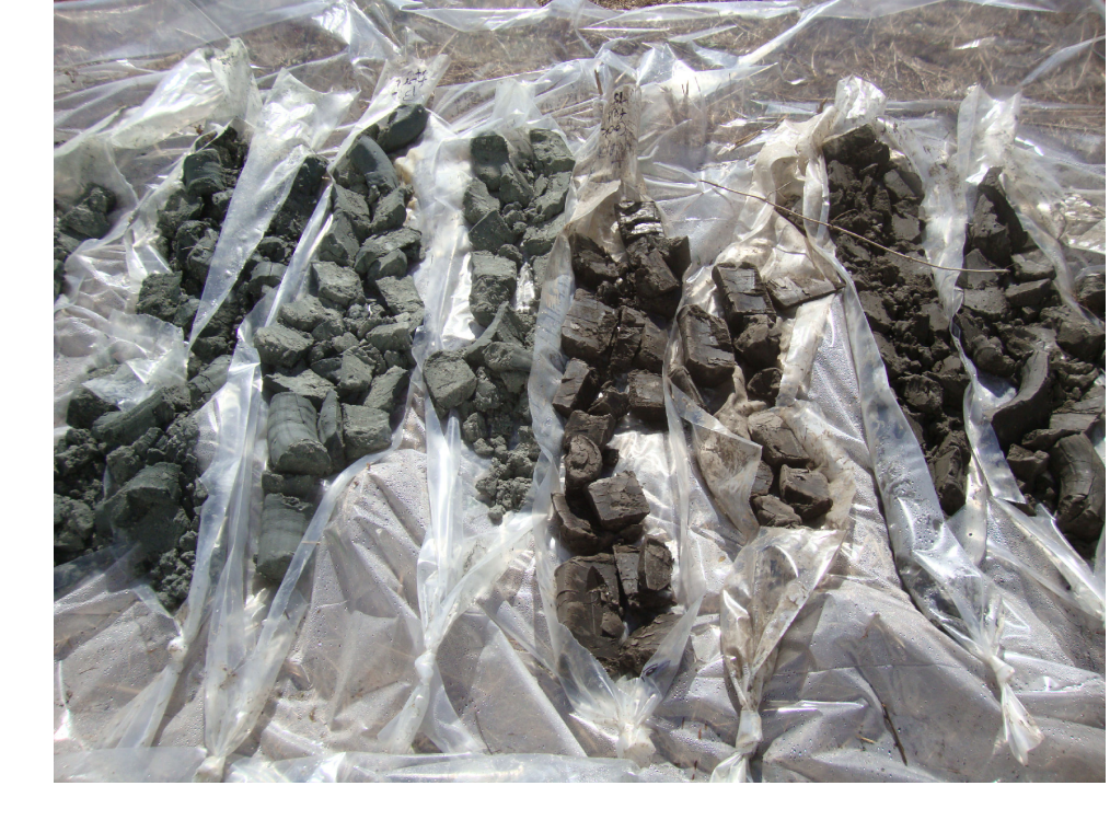
Core samples through the unconformable contact of Eocene glauconitic marine sandy marl of the Moody's Branch Formation at left (60-70 feet) with the underlying Eocene carbonaceous clays in the uppermost Cockfield Formation at right (70-80 feet). Photographed on November 7, 2012, in Section 19, Township 9 North, Range 3 East.
