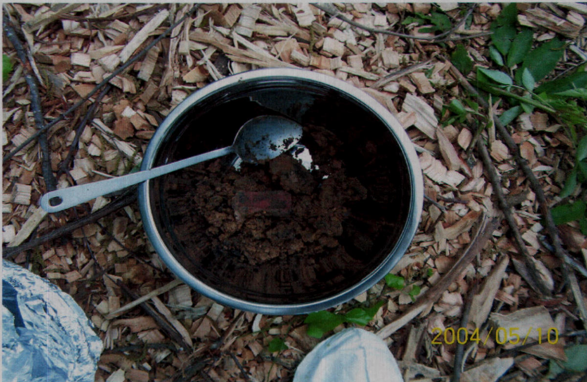
PHOTO 15 – A view of a typical sample taken from the trackhoe bucket during installation of the test pits. Note brick debris and discolored soil.
