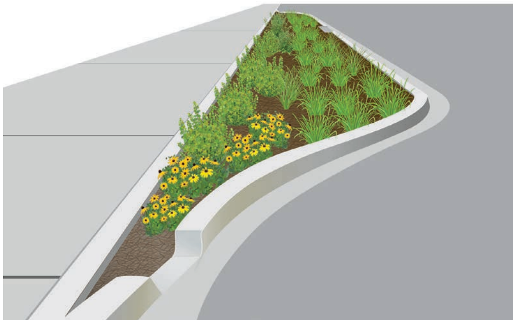
Figure 5-4. Example of a rain garden configured as a curb extension to capture street runoff.
