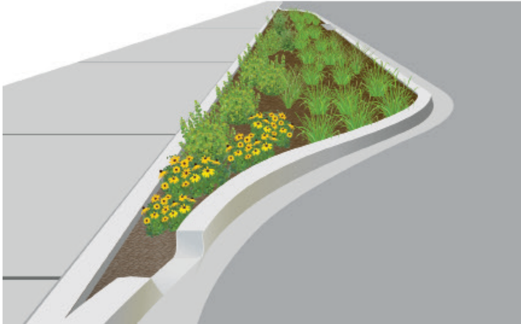
Figure 5-4. Example of a rain garden configured as a curb extension to capture street runoff.
